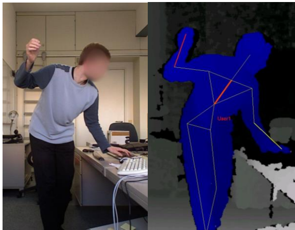
Figure 3: Left: Colour image of a subject. Right: Depth image and the tracked skeleton. The system draws the back bone and the right arm in red since they represent two examples of ergonomically unfavourable poses.
