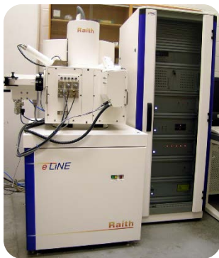
Electron-beam lithography system and example pattern (magnetic quasi-crystal)
